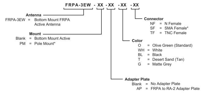
Note: SMA connector is not recommended for use with LMR400 cable. \*Adapter plate and pole mount can not be ordered together in a single configuration.
